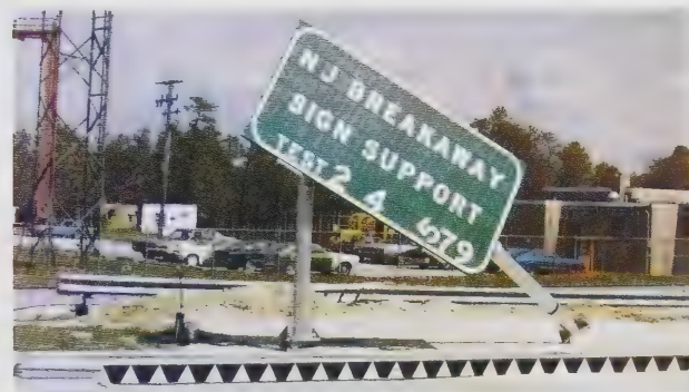
The breakaway coupling for large highway signs developed by NJDOT Engineer Richard A. Strizki . (1969)
